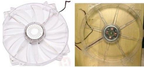
Figure 4. a) 20 cm DC12V 0.30A LED computer fan b) The skeleton of the fan with the original blades removed
