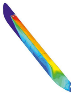
Fig. 4 "CFD simulation of a single chamber air cavity for a tanker"
