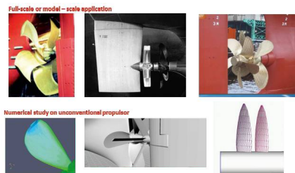
Fig. 7 "Typical Energy Saving Devices used in TARGETS"
