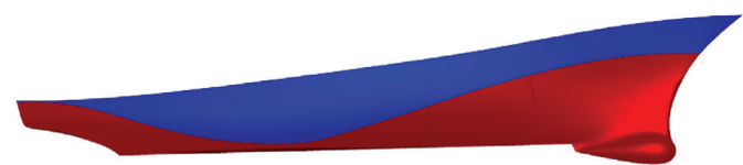
Figure 2. View of the DTMB 5512 when the ship is on the wave trough
